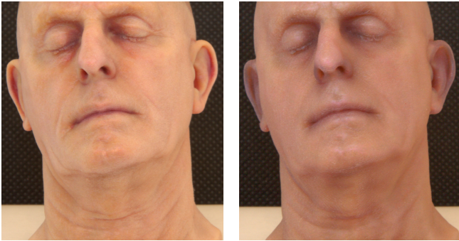
Fig. 11. Head model printed with relative \alpha = 1 (left) and \alpha = 0.5412 (right). Identical model geometry and illumination conditions.
