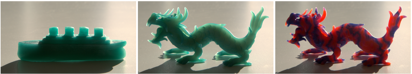
Fig. 14. From left to right, illuminated from behind by daylight: A ship figurine sculpted out of green wax, a 3D printed dragon with color and \alpha measured from the same wax, a 3D printed dragon with the same \alpha , but a fractal noise pattern for color, simulating a mix of red and blue waxes.
