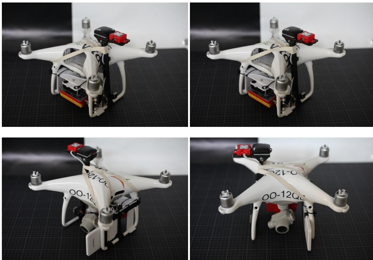
Figure 6 Final result of the integration of the MicaSense RedEdge-M under the Phantom DJI 4 pro.
