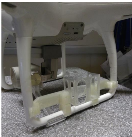
Figure 1 Mounting bracket for the STS-VIS attached to the DJI Phantom
