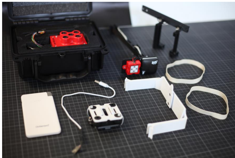
Figure 5 Materials needed to integration the MicaSense RedEdge-M under the Phantom DJI 4
