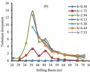
Fig. 12 Turbulent dissipation at different levels in USBR II stilling basin with end adverse slope—(a) RNG Model, (b) K-Epsilon Model
