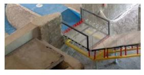
Fig. 1 Hydraulic model of Nazloochay dam
