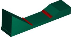
Fig. 5 USBR II stilling basin with end adverse slope
