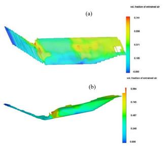
Fig. 11 Simulation of Fraction of entrained air in USBR II stilling basin with end adverse slope– (a) RNG Model, (b) k-ε Model
