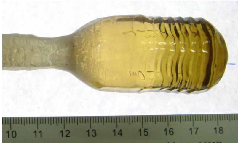
Fig. 3. Photo of as-grown YAG crystal.
