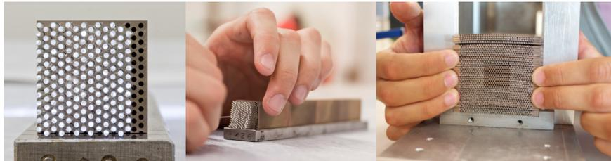
**Fig. 7.** Tungsten-Copper absorber units for electromagnetic calorimeter designs (left) and larger scale assembly with 9 sub-units. Each unit can be filled with various fibre-shaped materials: Cerium-doped silica glasses (as illustrated here), DSB fibres or also YAG:Ce crystal fibers.
