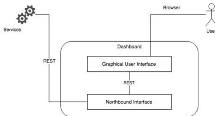
**Figure 13: Dashboard High Level Architecture**
