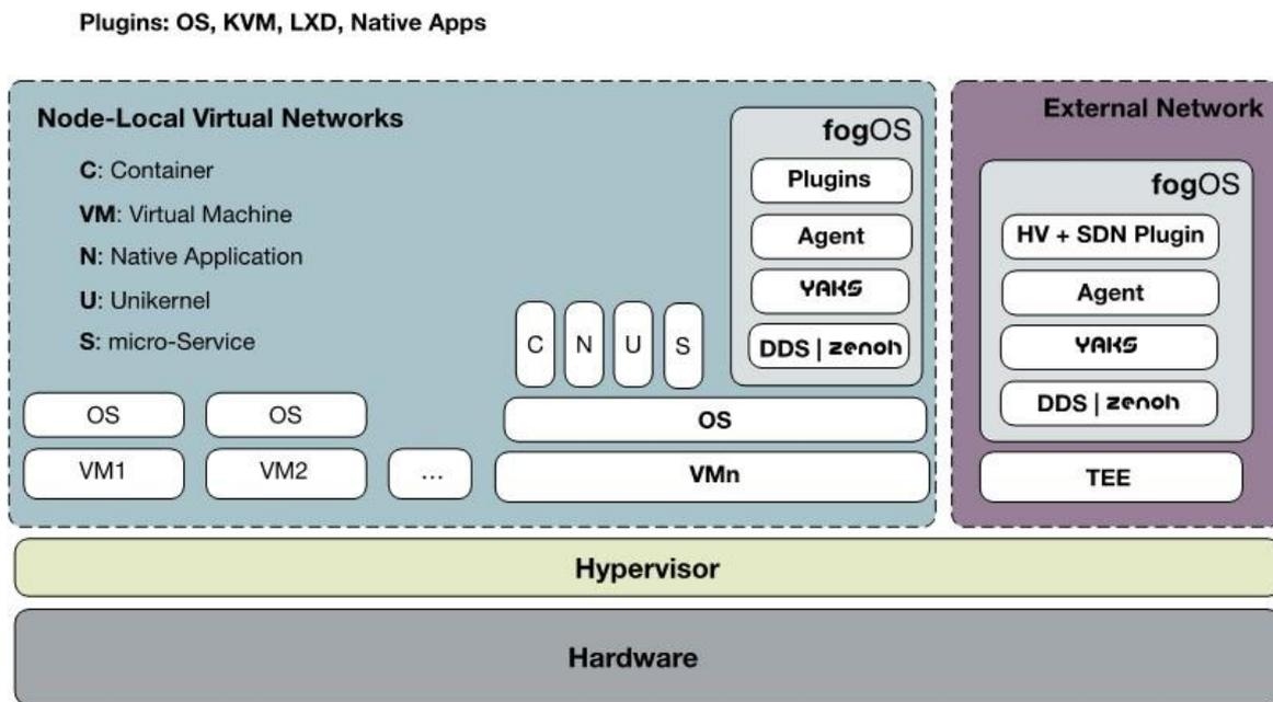
**Figure 18: The High-level architecture of Fog05**
