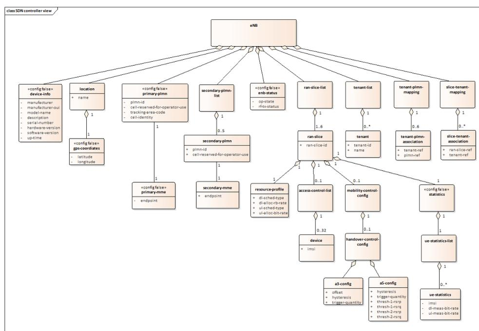
Figure 30: RAN SDN Control Interface Model
