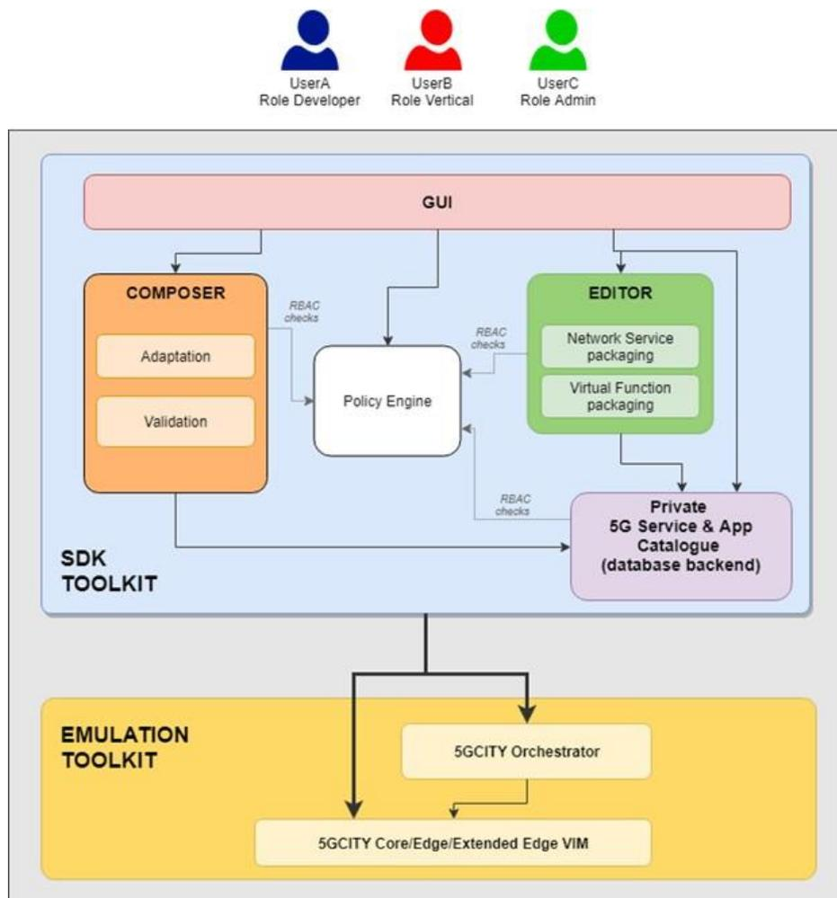
Figure 9: SDK Toolkit high-level architecture.
