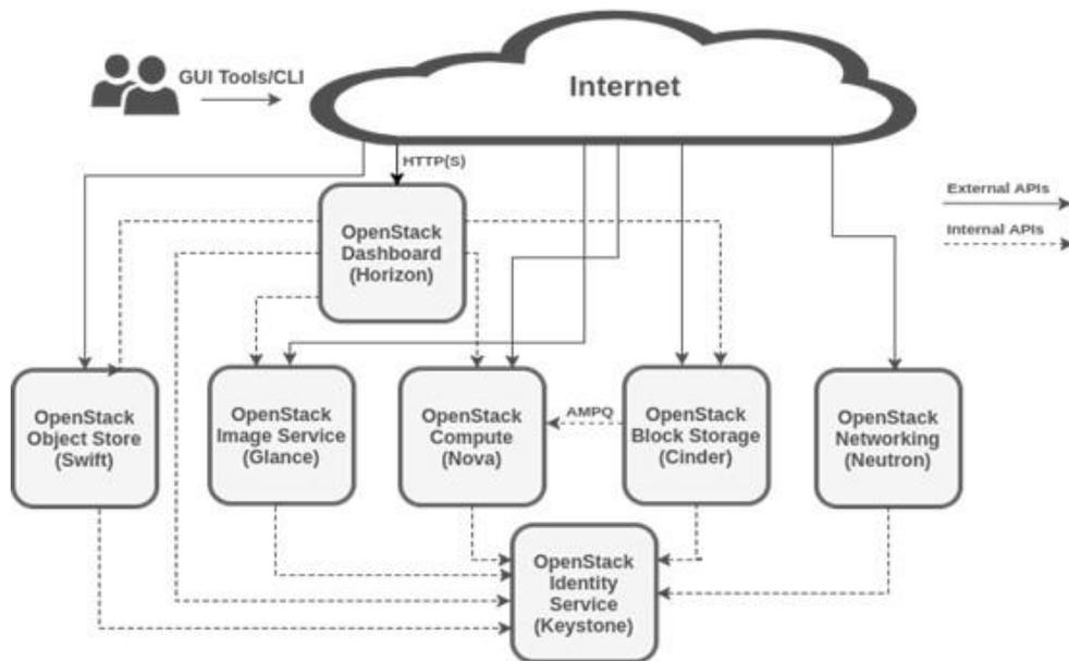
**Figure 15: OpenStack architecture**
