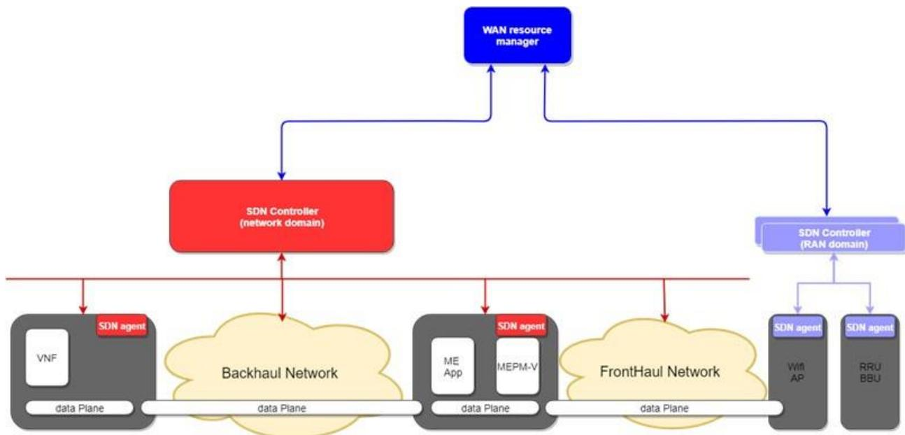
**Figure 20: SDN Controllers on 5GCity architecture**
