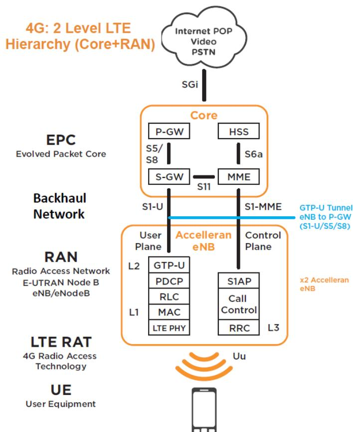
Figure 31: 4G - 2 Level LTE Hierarchy (Core+RAN)
