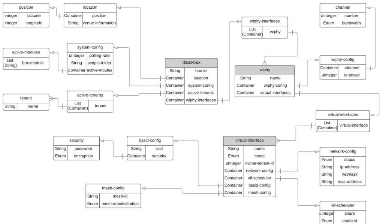
**Figure 22: Wi-Fi node Yang control interface model**
