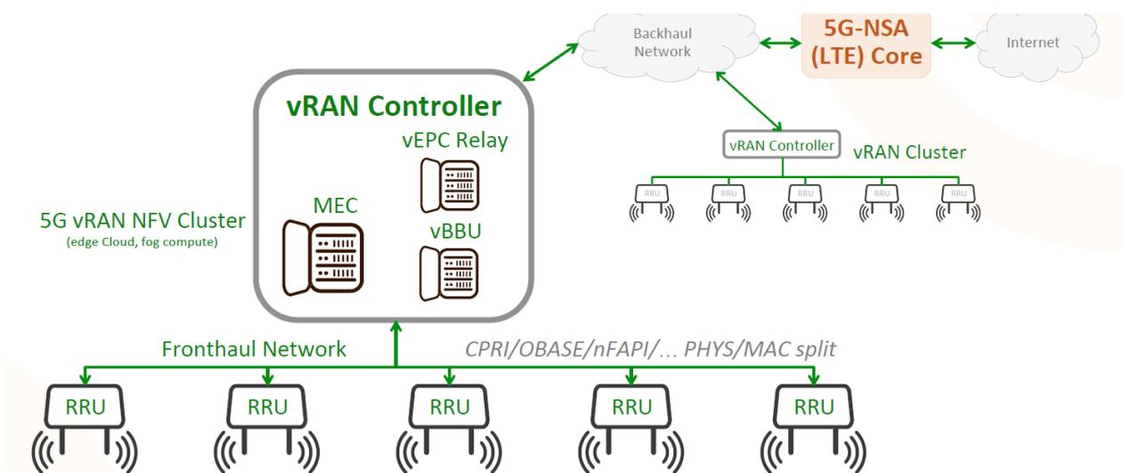
Multi-RAT 5G-NR/LTE-A, Massive MIMO beamforming, 'Cluster SON', sub 6 GHz – mmWave
