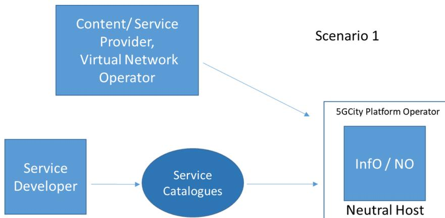
**Figure 4: Scenario 1: Infrastructure Owner and Network Operator collapsed in one role**
