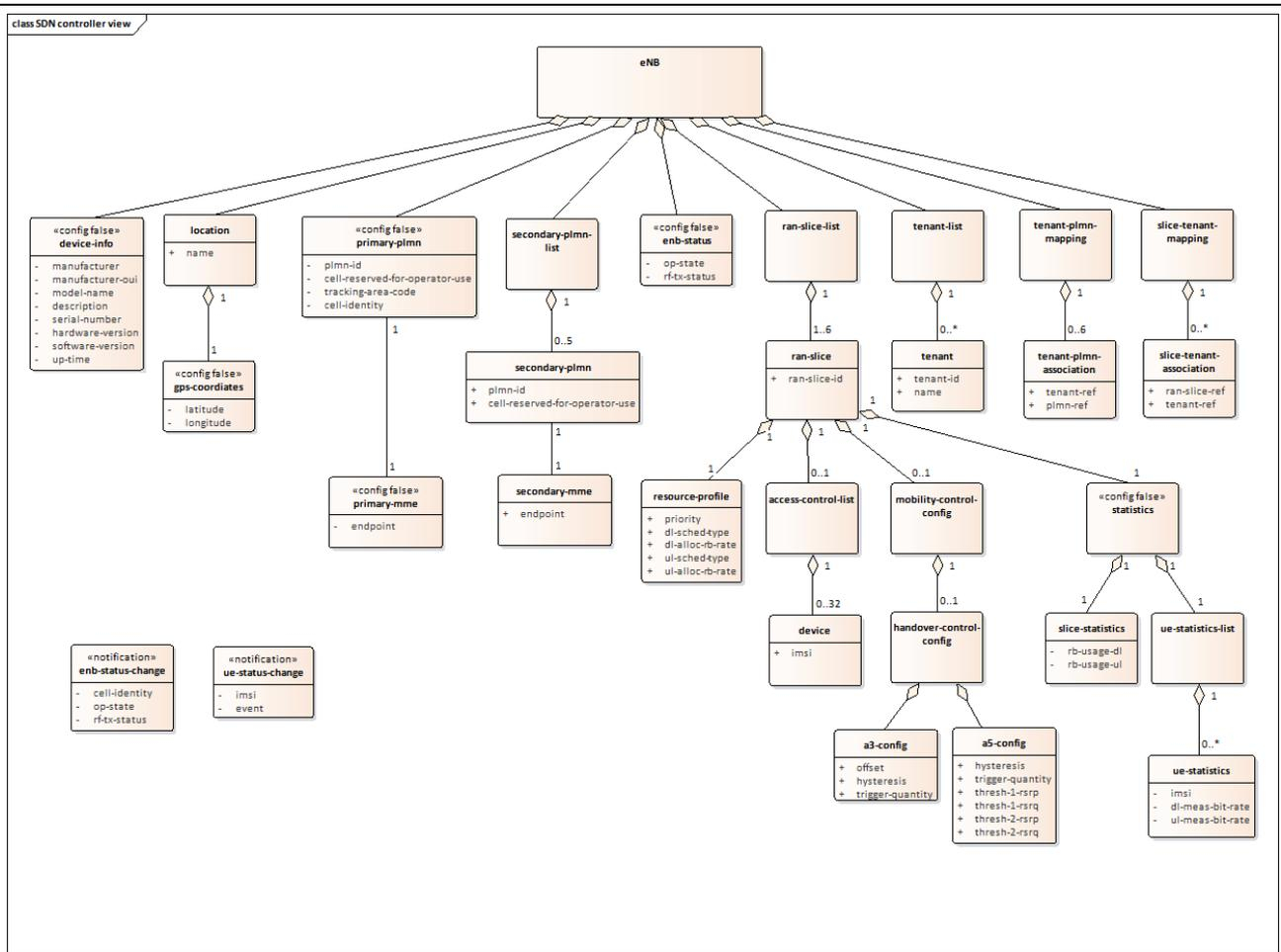
**Figure 23: RAN SDN Control Interface Model**
