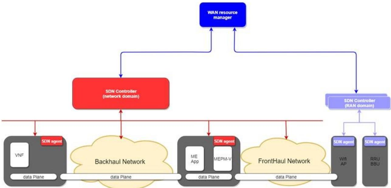
**Figure 20: SDN Controllers on 5GCity architecture**
