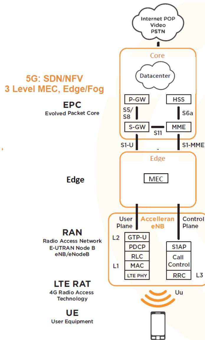
Figure 32: 5G - SDN/NFV 3 Level MEC, Edge/Fog
