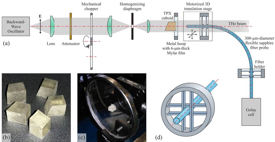
**FIG. 3.** Experimental setup for visualization of the PH relying on principles of the scanning-probe THz imaging and exploiting a flexible 300- $\mu\text{m}$ -diameter sapphire fiber: (a) a scheme of the experimental setup; (b) a photo of the TPX cuboids; (c) a photo of the TPX cuboid glued onto a 6- $\mu\text{m}$ -thick Mylar film mounted on a metal frame; (d) a scheme of the sapphire fiber handling using crossed polymer cords.
