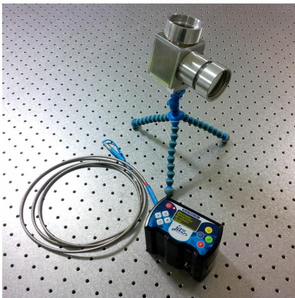
Figure 1: The spectrograph, the optic fiber and the light collector used to take spectra during fieldwork.
