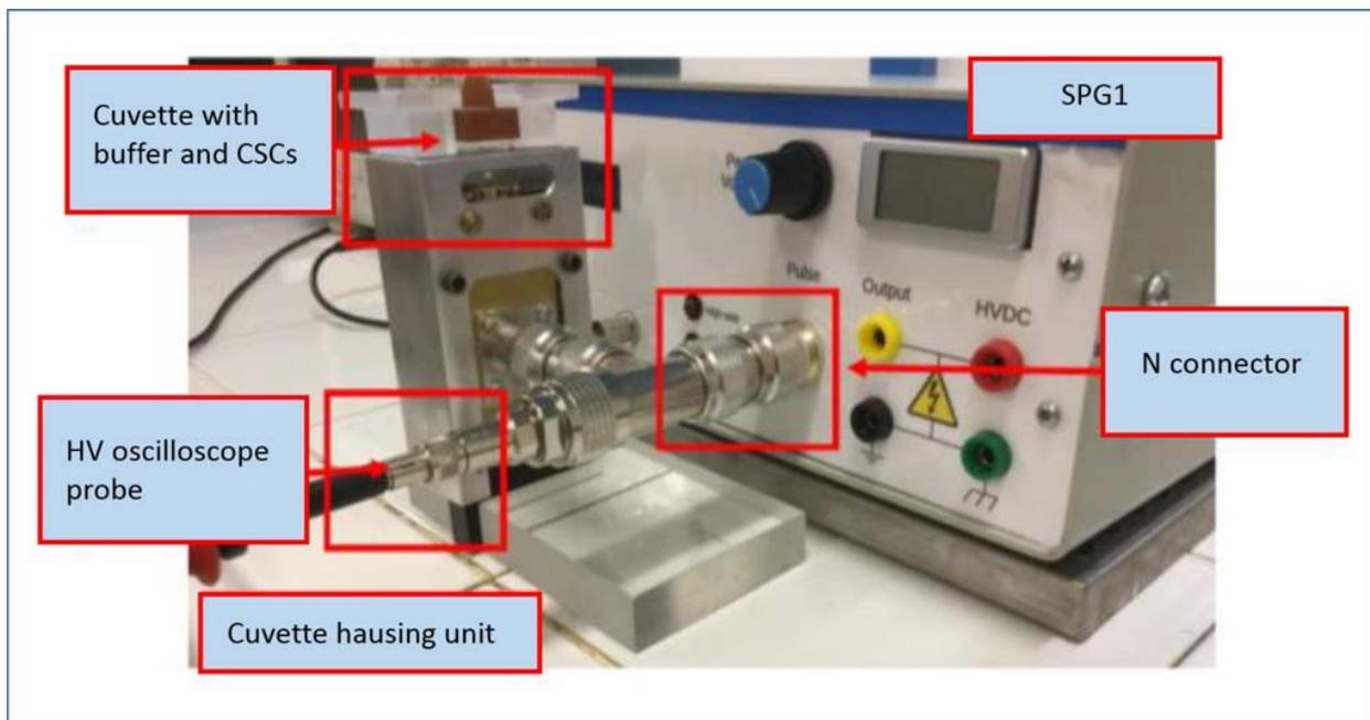
Figure 1. Instrumentation setup: the SPG1 generator, the cuvette housing unit filled with a 50 ohm buffer and CSCs
