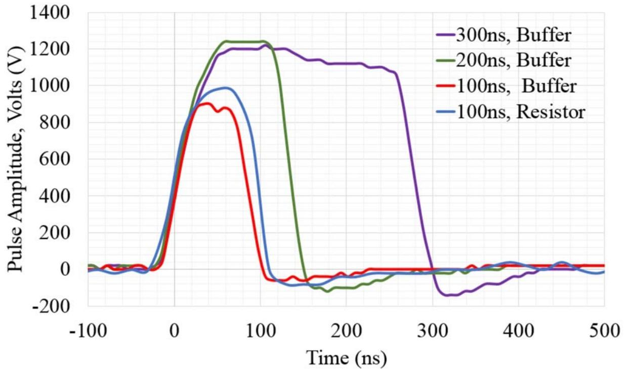
Figure 2. 100 ns, 50 Hz, 20 burst waveform, with 50  $\Omega$  resistor as SPG1 load (blue). And 100 ns (red), 200ns (green) and 300 ns (purple) pulse, 50 Hz, 20 bursts waveform measured with CSCs in the 50  $\Omega$  buffer load.
