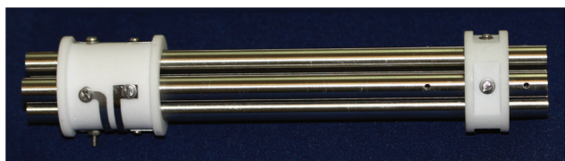
Fig. 2 Optimized dual filter quadrupole analyser assembly with circular rods manufactured using CNC machining and integrated in the portable MS system. r_0 = 2.76 mm, rod diameter 6.35 mm, pre-filter length 22 mm, and main filter length 110 mm.
