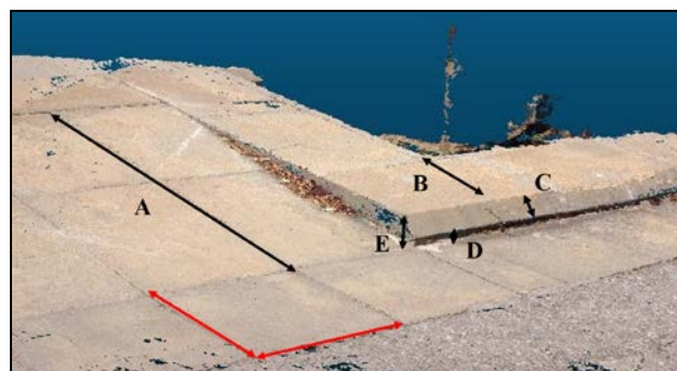
Figure 7. Curb ramp scenario. 3D reconstructed point cloud along with reference targets. The measurements used to compute the point cloud are represented in red, while the reference measurements used to check the relative accuracy of the point cloud are represented in black.
