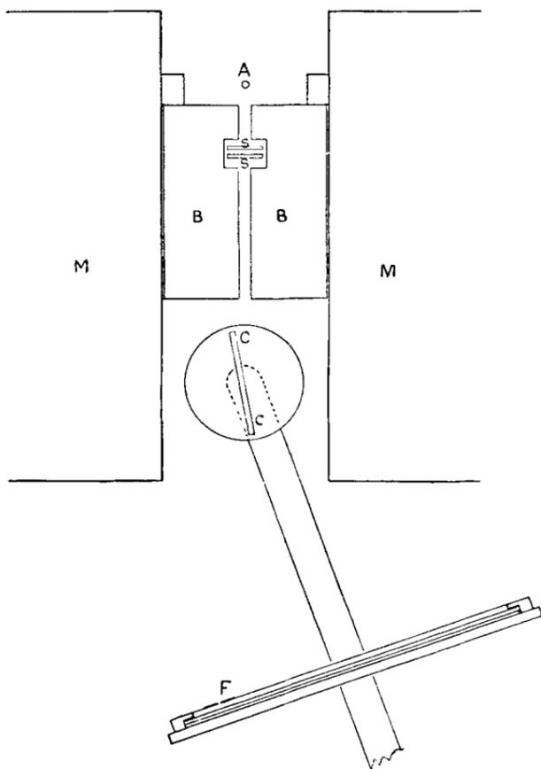
the rectangular pole-pieces of a powerful electromagnet *MM*, as indicated in the diagram; the magnetic field usually employed was 2500 gauss.
