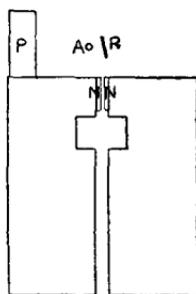
from it could strike the photographic plate. A second block of lead P was placed behind it, to increase the intensity by means of successive "reflexions" of the  $\beta$  rays between this block and R.
