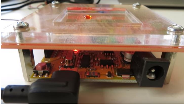
Figure 15: Side view of the real-biochip moving a droplet.
