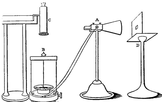
The heated body is placed behind the diaphragm, filling up the field of view from the cone; so that every ray reaching the cone from behind the diaphragm comes from the heated body.
