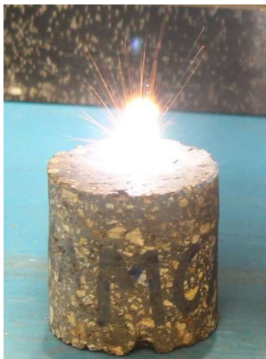
Figure 5 – Refractory sample with plasma from the LIBS-system
