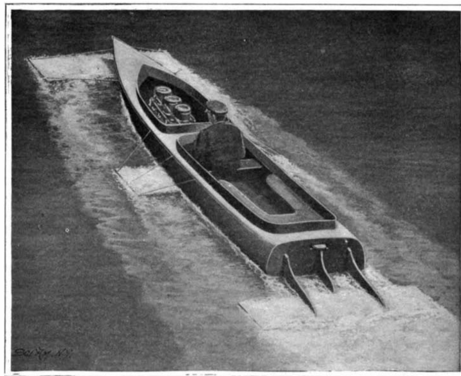
Motor Boat Fitted with Three Surface Hydroplanes of the Type Proposed by Archdeacon.
