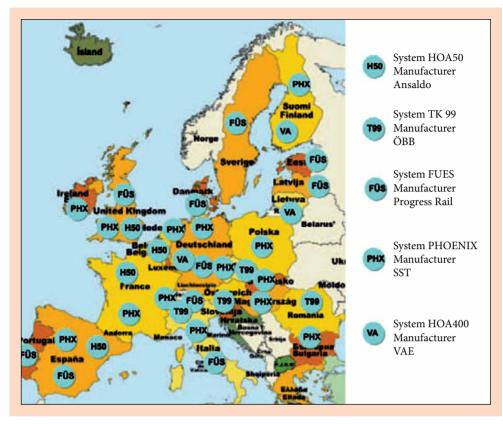
Figure 10. Hot axle-box detection systems in Europe Railways (Eisenbrand 2011)
