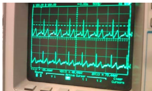
Fig. 7 Typical recordings from ECG Electrodes shown on the oscilloscope. The same can be obtained on laptop, or microcontroller or smart phone display for sending to the medical expert
