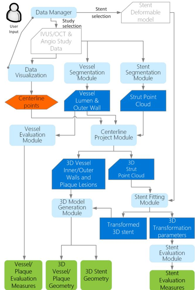
Figure 2. Information flow of 3D reconstruction and plaque characterization tool (IVUS/OCT case).
