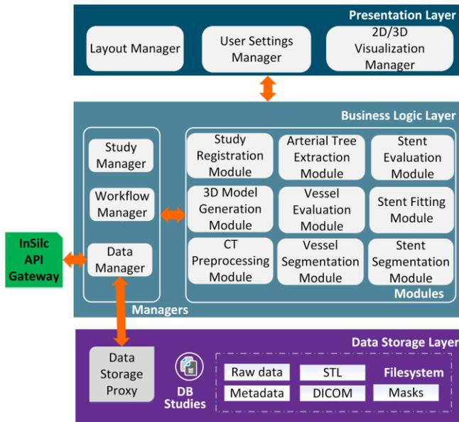
Figure 1. Detailed architecture of 3D reconstruction and plaque characterization tool.
