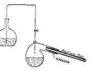
inum condenser is provided with a short glass cooler, leaving about 20 cm. of the upper end free. About 15 cm. of this free end extends into the neck of a 4-liter retort, and the space between the platinum and glass is packed with asbestos. By this arrangement *only the water which is condensed in the platinum tube is collected*, while the water which condenses in the neck of the retort drips out at the asbestos packing.
