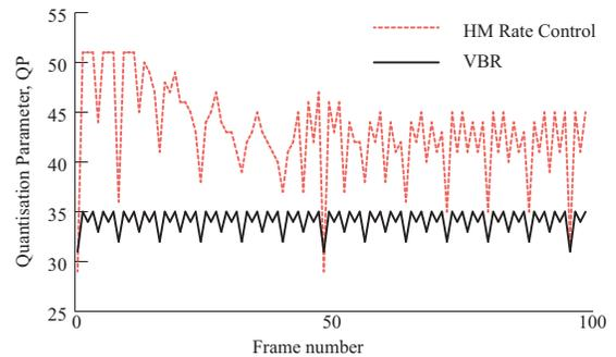
Fig. 1. QP values for the first 100 frames of the *Somersault* test sequence which correspond to the rate obtained with QP value 31 for VBR. QP values associated with VBR encoding are denoted with black, while QP values used by the rate control in HM are depicted with a red dotted line.
