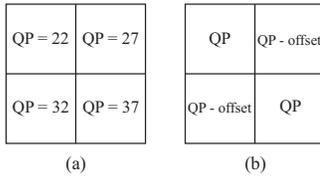
Fig. 3. Variable QP pattern used within a frame for (a) intra frames, (b) inter frames. Each square represents one CTU.
