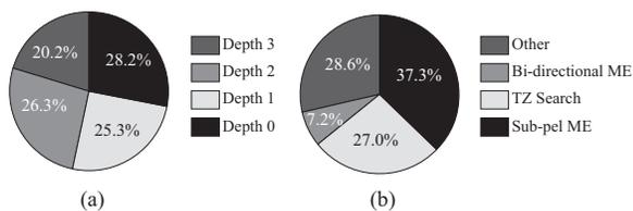
Fig. 2. *HM-fast* encoder profiling: (a) percentage of encoding time spent on each CU depth and (b) percentage of time spent in each module for depth 0.
