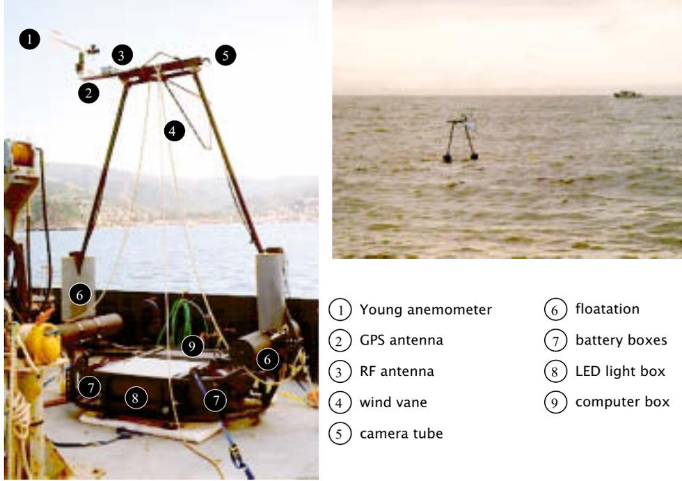
Figure 3: Instrumentation to take image sequences of the slope of short wind waves at the ocean interface as an example of a passive tracking system. Left: Wave-riding buoy at the stern of the RV New Horizon. Right: deployed buoy. Almost all parts of the buoy including the light source are submerged.
