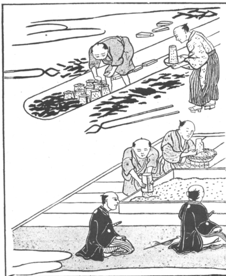
Fig. 3. Charging the furnace. Japan.
