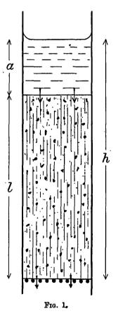
If we consider a vertical tube of soil (Fig. 1), of length l, through which water is flowing under the influence of a head of pressure a + l = h, and escaping freely at the lower end; then
