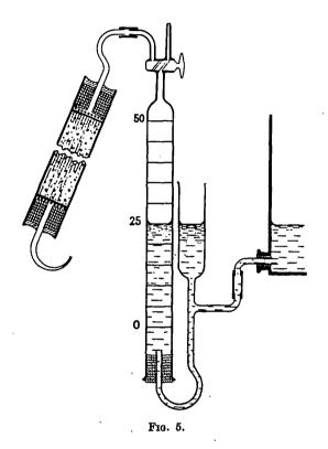
The observations recorded in Table V. were taken with both "head" and "tail" of pressure on a tube filled with loam.
