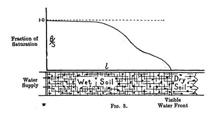
If we assume that the water present in this region is distributed uniformly among the fine and coarse capillaries then the average effective length of the soil column will be equal to  $\frac{v}{AS}$ , the volume of water which has entered the tube per unit area of cross-section of the soil pores. But  $\frac{v}{AS} = \frac{m}{sAS}$  where m = the mass of water absorbed by the soil column, and s = density of water = 1 (with sufficient accuracy).
