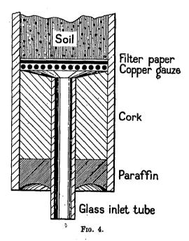
§ 21. Procedure recommended for the "physical examination" of soils.—In later experiments weighings were taken not only of the soil used but also of the water absorbed, and the following method of procedure was adopted for the "physical examination" of soils:
