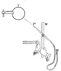
A tuning fork held in one hand is made to touch the lath held in the other while vibrating, and the whole moved nearer to or further from the tambourine.
