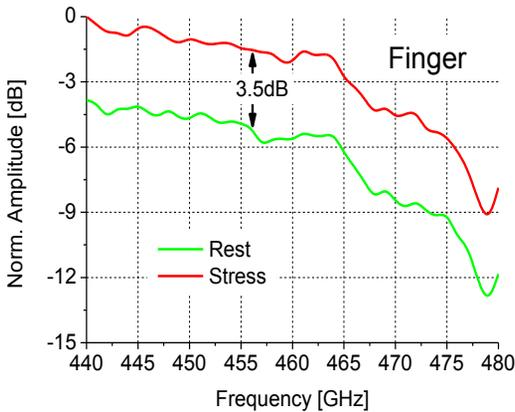
Figure 10: Skin reflectance in hand under rest and mental stress in Band-II
