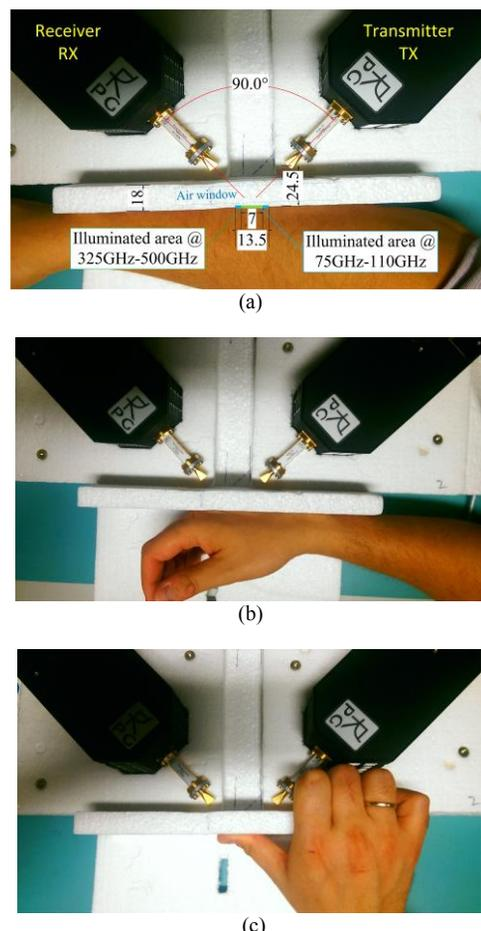
Figure 3: Measurement hand locations
