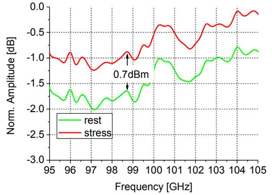
Figure 6: Skin reflectance under rest and mental stress in Band-I
