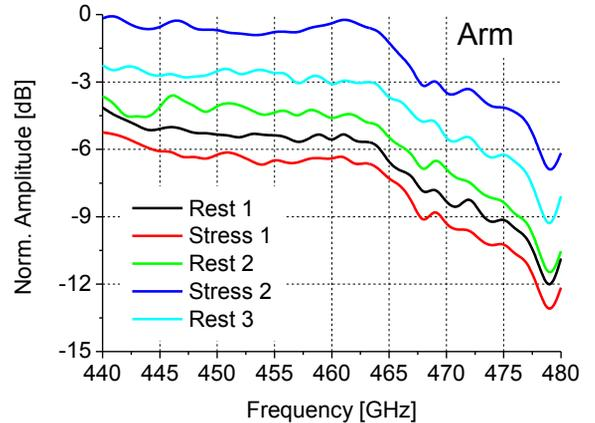
Figure 8: Skin reflectance under rest and physical stress in Band-II
