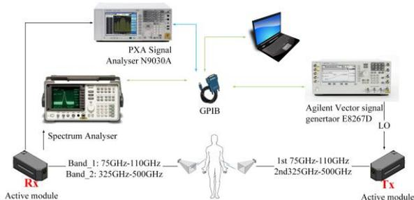
Figure 2: Skin reflectance measurement setup.
