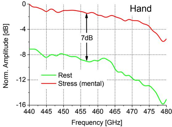
Figure 9: Skin reflectance in hand under rest and mental stress in Band-II
