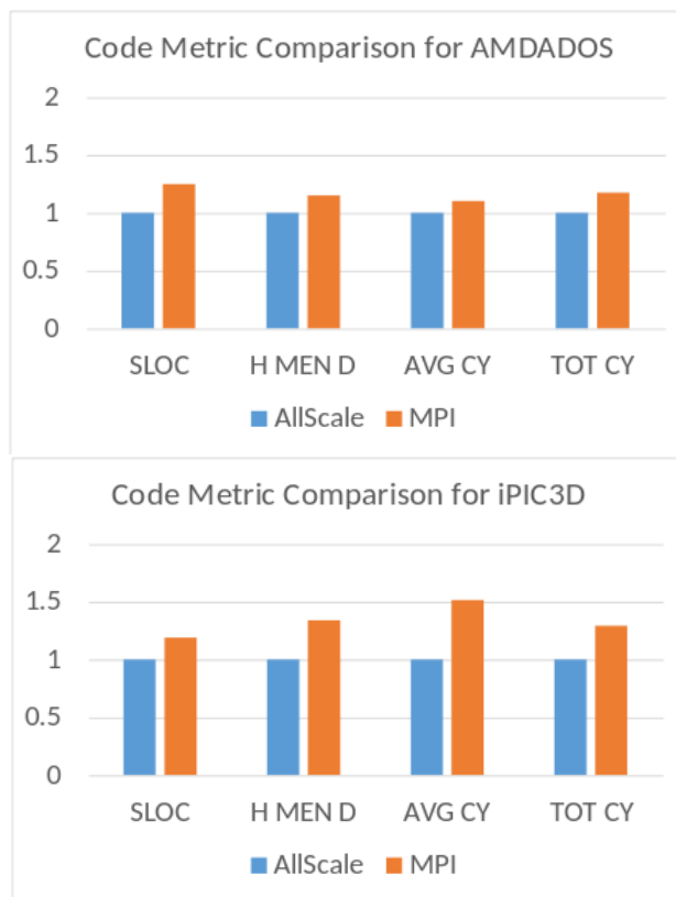
Figure 3: Code metric comparisons for AllScale and MPI implementation of pilot applications. The y-axis represents each metric normalised to the AllScale implementation (i.e. AllScale metric = 1.0 for each metric)
