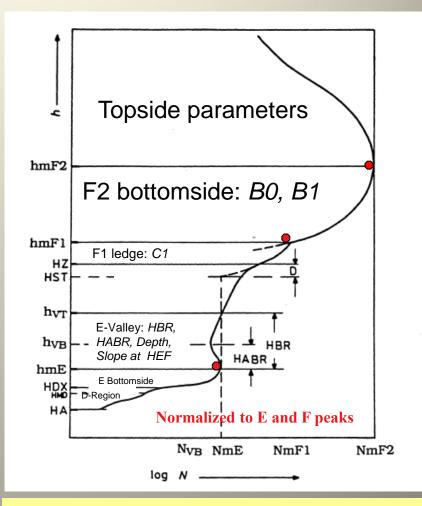
Global models for anchor points: foF2/NmF2 foF1/NmF1, foE/NmE, foD/NmD, hmF2/M(3000)F2, hmF1 , hmE, hmD
