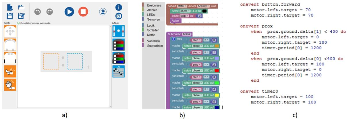
Fig. 2. Programming languages available in Aseba Studio. a) Visual programming. b) Blockly programming. c) Text programming.
