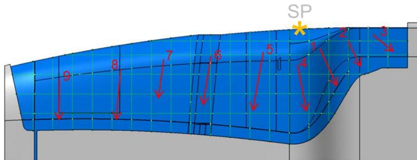
Fig. 4: Principle of the manual draping process, as an illustration of the force application steps
