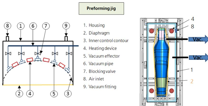
Fig. 9: Design of the compacting unit [3]
