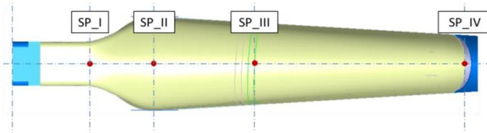
Fig. 2: Predefinition of four possible initial draping points on the top of the tooling
