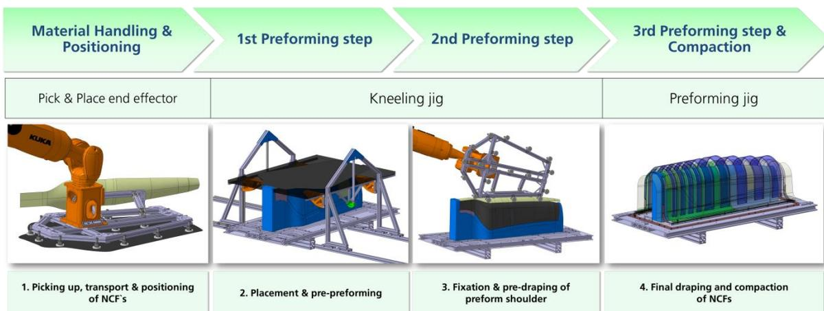
Fig. 5: Process sequence in four steps
