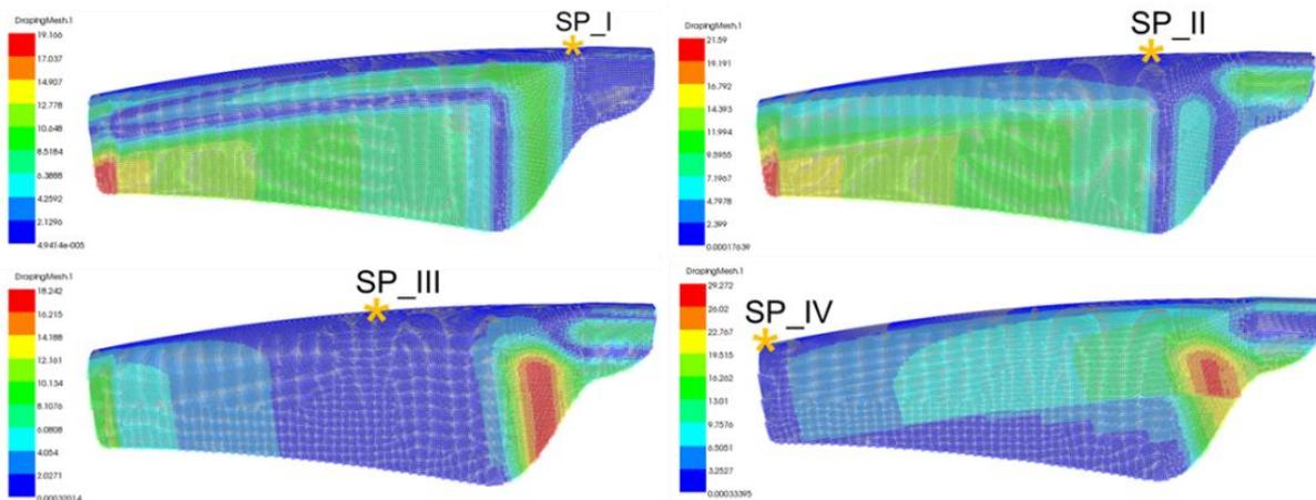
Fig. 3: Shearing effects based in location of initial draping point [1]
