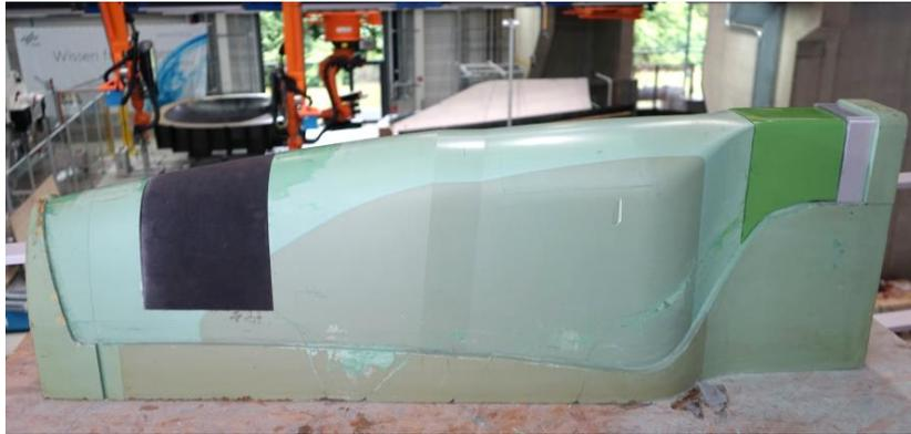
Fig. 1: Male AFS Tooling used for the development of an automated preforming process
