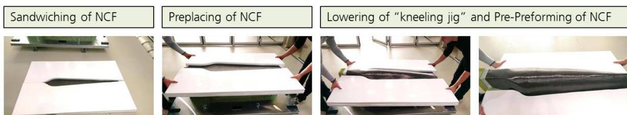
Fig. 7: Preliminary test of the deposition of cut-pieces with the clamping method
