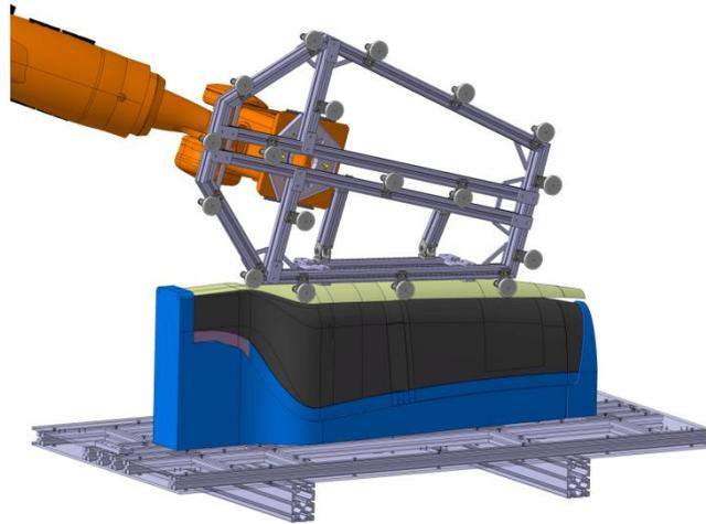
Fig. 8: Pre-fixation und compaction of the preform using a caul plate
