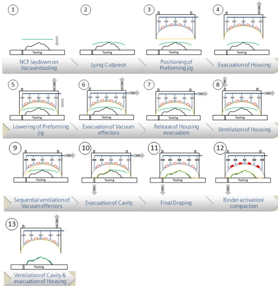
Fig. 10: Sequence of the automated drape and compacting process [3]
