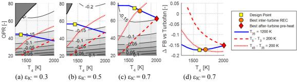
Fig. 10: (a-c) Fuel burn parameter studies for CCE with IC before PC for various  $\varepsilon_{IC}$  from 0.3 to 0.7, and (d) fuel burn comparison for  $\varepsilon_{IC} = 0.7$ .
