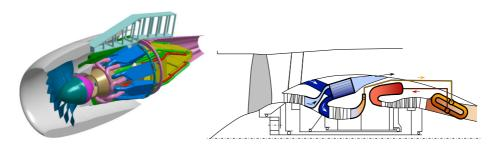
Fig. 2: The IR turbofan engine concept, developed by MTU Aero Engines [10].
