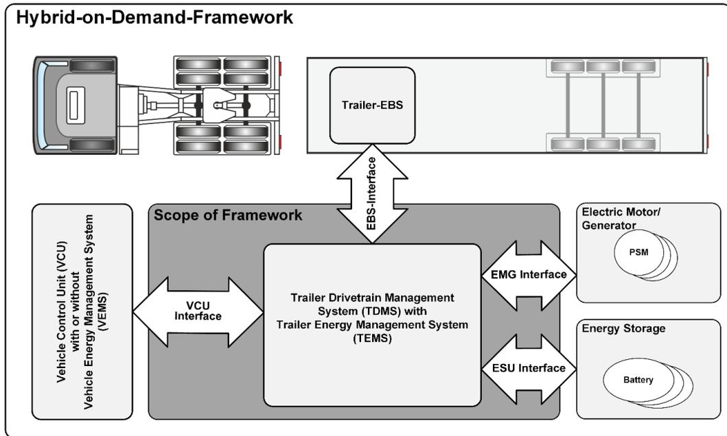
Fig. 3 Logical System Architecture of the HoD-Framework
