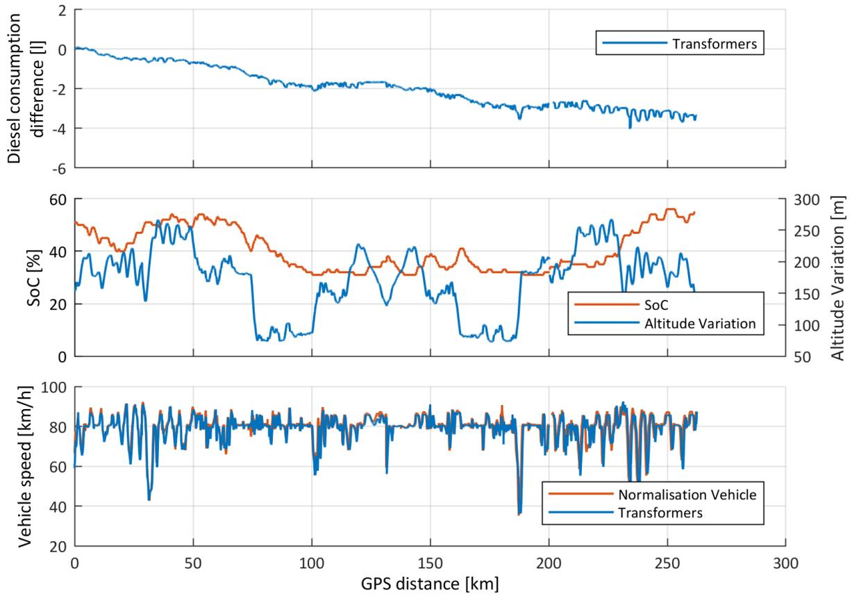
Fig. 6 Illustration of HoD operation; BOB test with 40 tonne GCW; speed profile mean standard deviation between normalization vehicle (Ref FH1758) and the Transformers vehicle under test:  $\sigma = 1.5$  km/h
