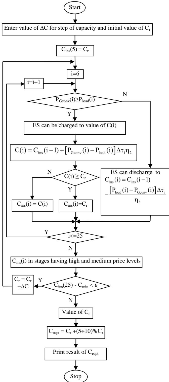
Fig. 5 Algorithm to determine optimal sizing of ES
