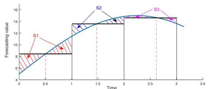
Fig. 2 Technique of area approximation to create rectangular diagrams
