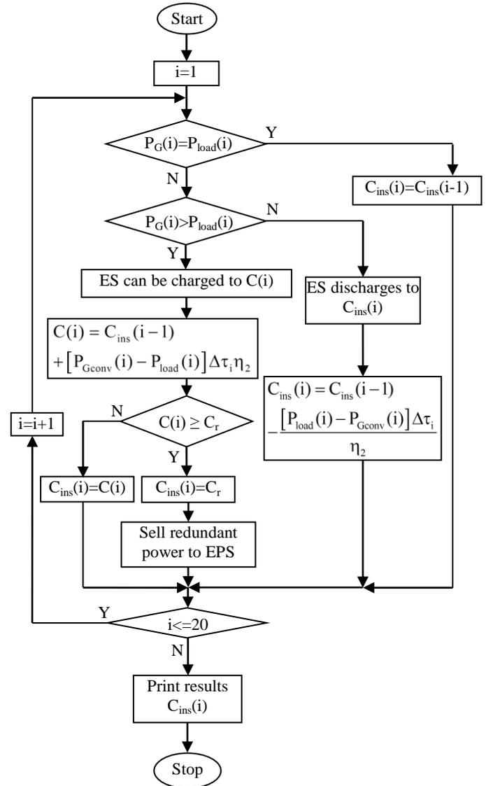
Fig. 6 Determine  $C_{ins}(i)$  in stages having high and medium price levels
