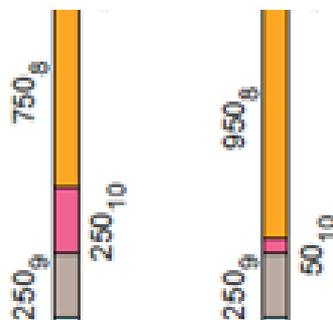
**Figure 2.** Inner/outer (left/right) FA axial layouts in the core and lower blanket, from bottom to the top: steel reflector of 250 mm (9), fertile blanket of 250/50 mm (10), fissile part of 750/950 mm (8)
