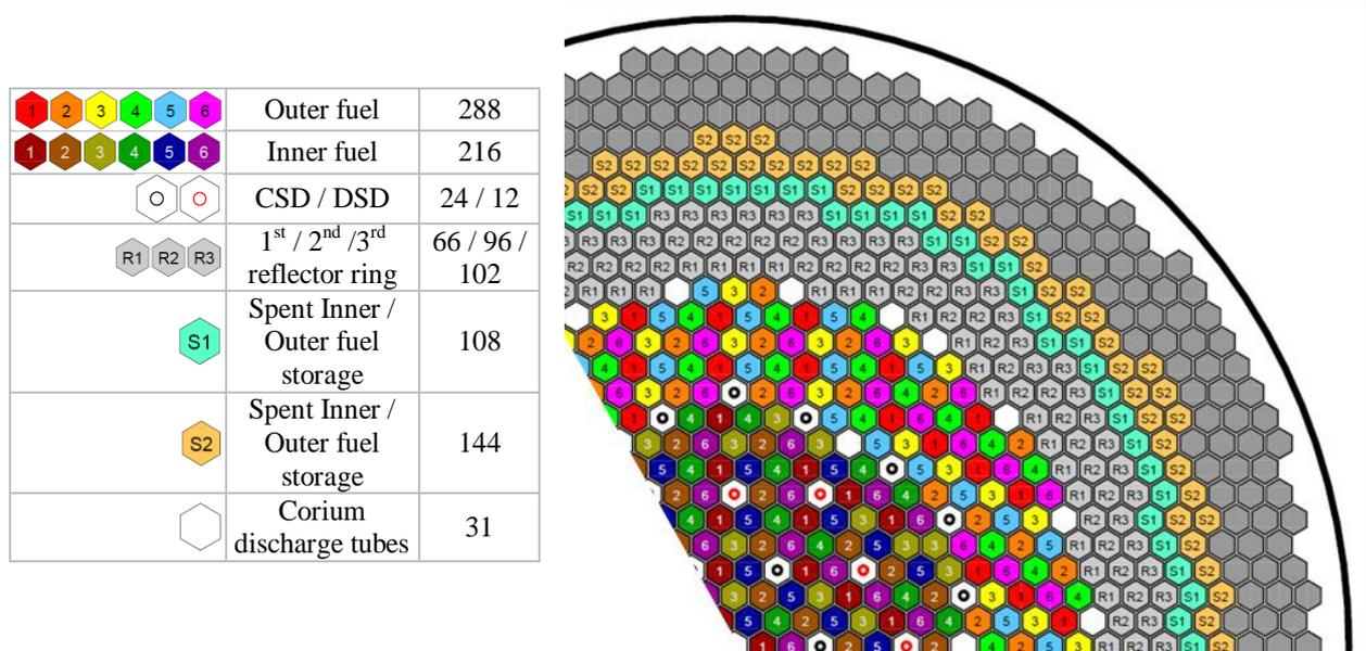
**Figure 1.** ESFR core layout in plane, the HEX pitch is 20.985 cm
