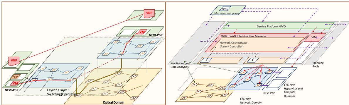
Fig. 1. (a) Metro-Haul Infrastructure, showing the main components: the disaggregated transport network interconnecting Metro-Haul locations (AMEN/MCEN nodes), the packet switched networks and the NFVI PoP encompassing computing, storage resources. (b) Macroscopic view of the Metro-Haul Control, Orchestration and Management (COM) and Service Platform, highlighting the NFV MANO part, the hierarchical SDN control, the Monitoring and data analytics (MDA) and Network Planning (NP) components
