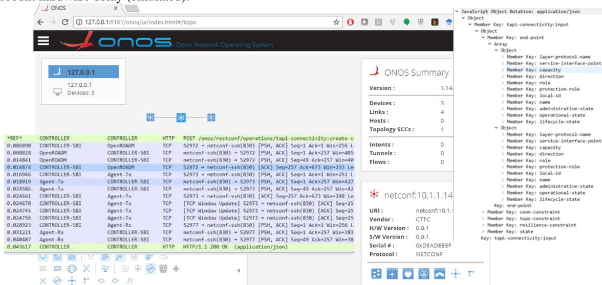
Fig.4. Experimental Validation of NETCONF/YANG device configuration after a TAPI NBI Request.
