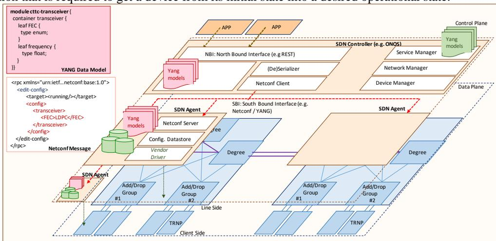
Fig.3. SDN Control of a disaggregated optical network (transceiver and/or optical line system)
