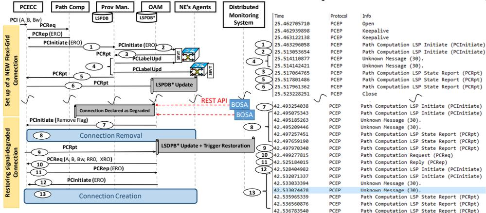
Figure 2. a. Workflow for restoring a signal-degraded connection; b. Captured PCEP messages
