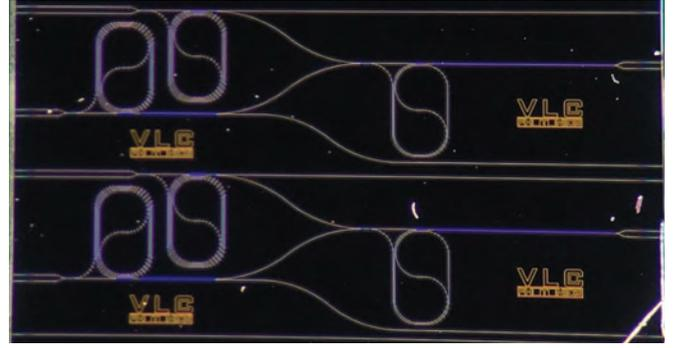
Fig. 2. PIC-based IDWPT/DWPT optical orthogonal transform processors corresponding to a 2-levels decomposition Haar wavelet
