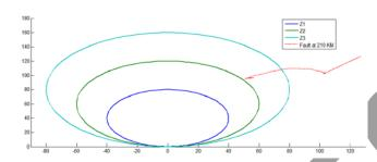
Figure 15.R-jX plot for a fault at 210 km distance Three Phase to Ground Fault (ABCG Fault
