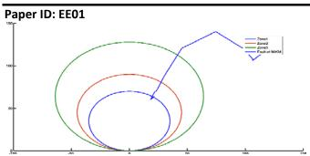
Figure 14. R-jX plot for a fault at 90 km distance
