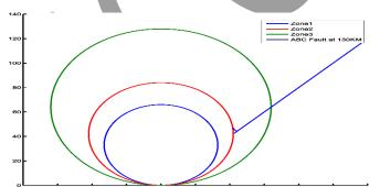
Figure 17.R-jX plot for a fault at 130 km distance
