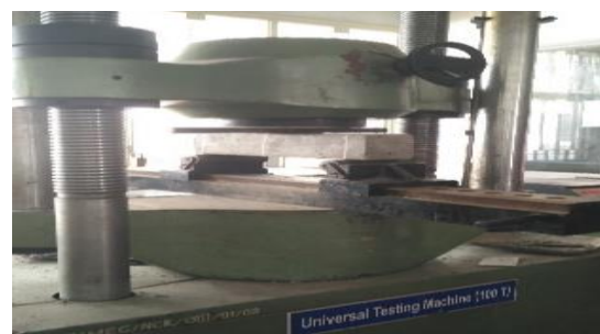
Fig: 5. Testing of Specimen for flexural strength
