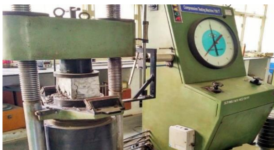
Fig: 3. Specimen failed due to compression
