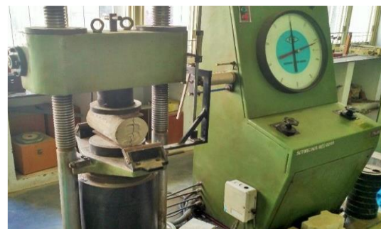
Fig: 4. Specimen failed due to splitting tensile test
