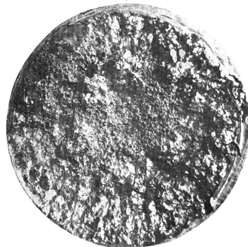
COPPER-ALUMINIUM STAY, BROKEN HEAD
