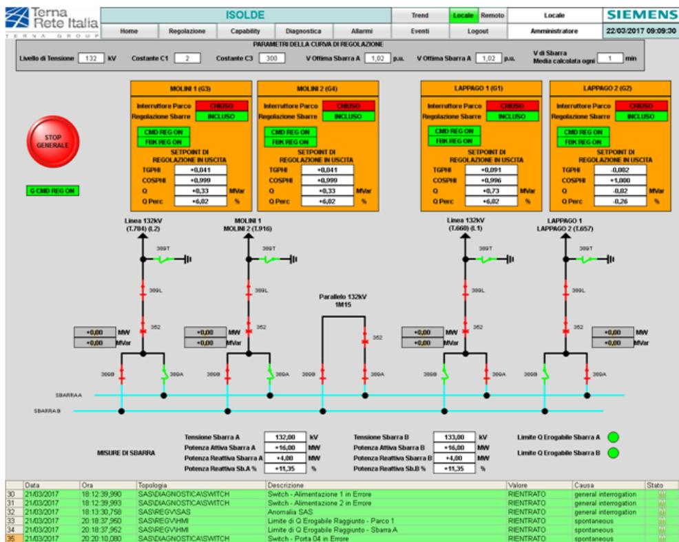
Figure 4 Main HMI of HVRS device
