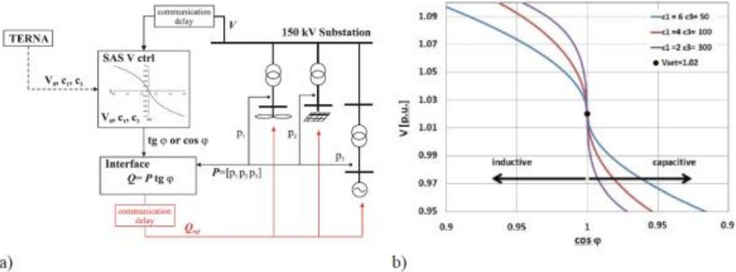
Figure 3 Proposed substation voltage control structure (left side) and control law (right side)
