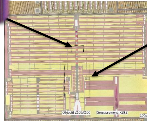
Prototype of microfluidic sensing platform on CMOS chip
