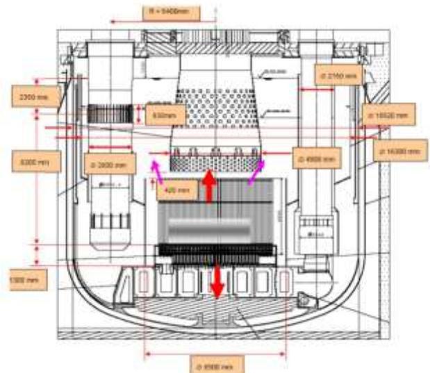
Fig. 1 ESFR Pool concept and potential relocation paths with geometrical values
