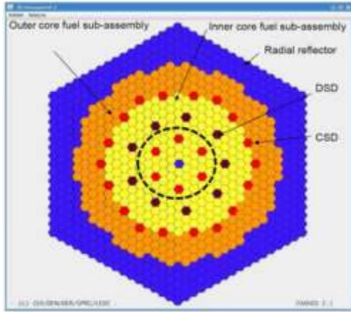
Fig. 2 Core layout of the ESFR reactor (7)
