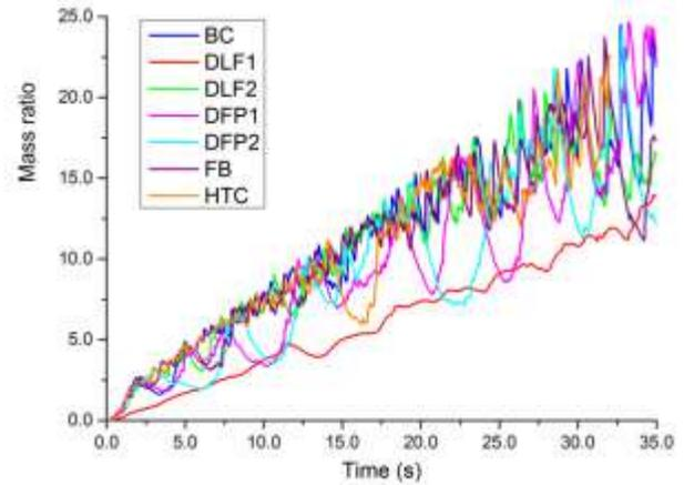
Fig 7 Mass ratio between fuel particle and liquid fuel
