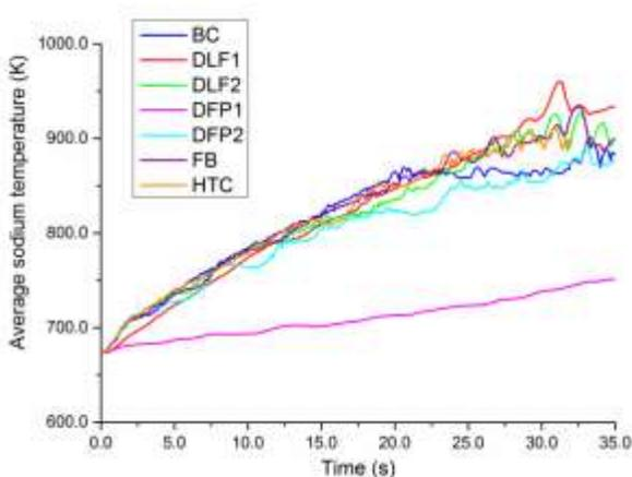
Fig 10 Average temperature of liquid sodium in the core catcher region
