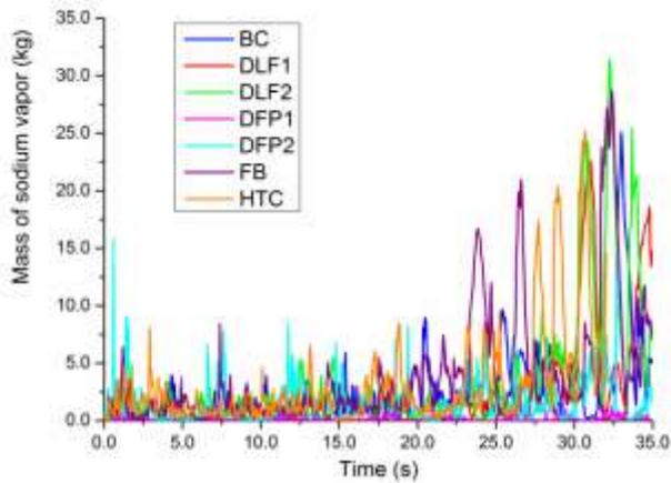
Fig 9 Mass of sodium vapor in the core catcher region
