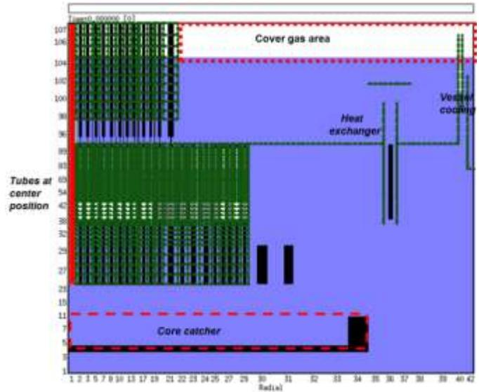
Fig. 3 simulation domain and initial position
