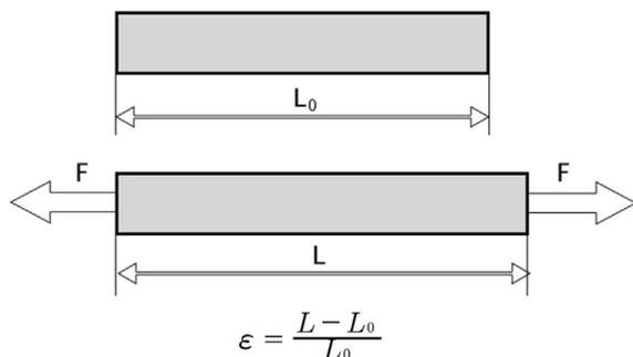
**Fig. 2** Tensile testing and strain calculation.
