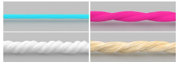
Figure 11: Renders of virtual replicas of the Gütermann swing yarns described in Table 3. From left to right, and top to bottom, the yarns are Skala360 (polyester), ORA 120 (polyester), CNe 50 (cotton), and S 303 (silk), with varying DoS.
