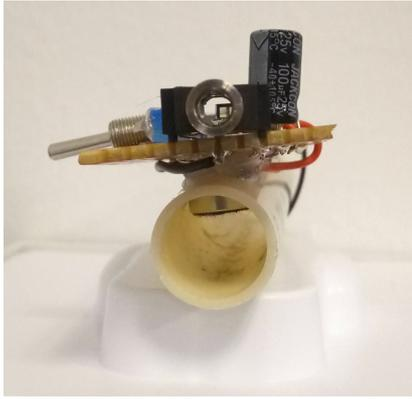
Figure 1: Wind instrument prototype (front view) consisting of an omnidirectional electret microphone (diameter = 0.8 cm); a 3 V button cell battery feeding the microphone with a supply voltage through a simple circuit; a plastic tube (length = 10 cm, diameter = 1.5 cm) with a round hole at 1 cm from the tail end, for flush-mounting the microphone.
