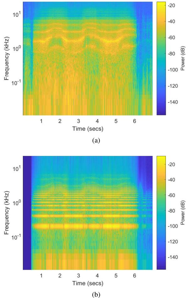
Figure 4: Spectral centroid scenario. The performer alternated between open ("a") and closed ("e") vowels, while blowing normally. The harmonic content of the output (4a) follows the input signal (4b).
