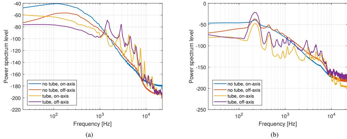
Figure 2: Power spectra of normal blows (a) and voiced blows (b) with/without the tube for on-axis/off-axis incidence.
