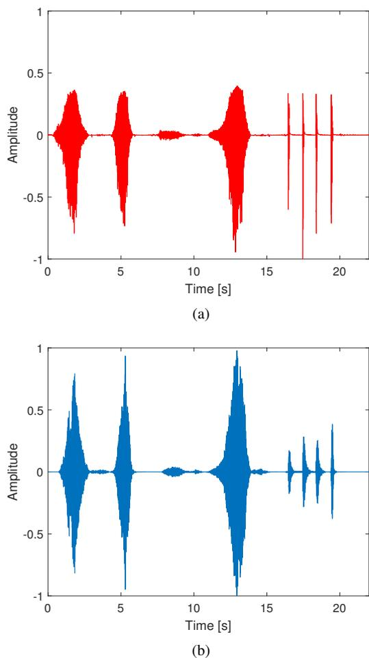
Figure 5: Envelope scenario. The performer sought to utilize different dynamics and durations, such as long/short, soft/loud, and abrupt/longer events, with no conscious vocal tract formation. The input signal is shown in 5a, the output signal in 5b.
