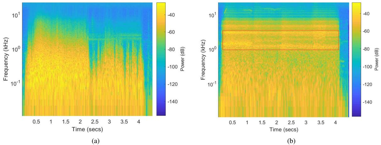
Figure 3: Spectrograms of varied vocal tract configurations for off-axis incidence, without the tube (a), and for off-axis incidence, with the tube (b). The red box highlights the region (around 2-4 kHz) where formants are emerging behind the standing-wave pattern.
