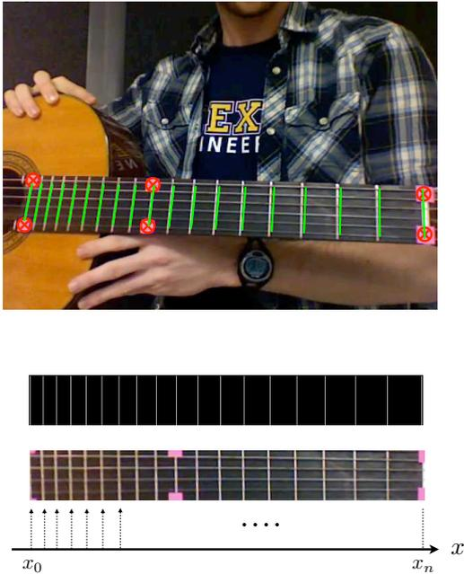
**Figure 4.** (top) Original image showing tracking points (in red), projected frets (in green) using the homography matrix. (bottom) Ideal fretboard, and subsection of original image after applying homography matrix to each coordinate.
