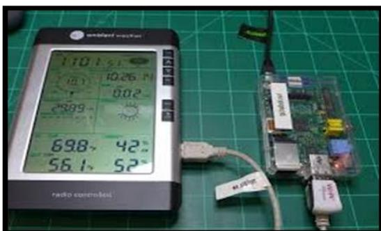
Figure 6: Weather Station on Raspberry Pi
