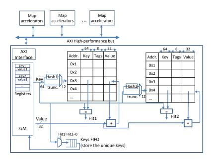
Fig. 5 Block diagram of the MapReduce accelerator
