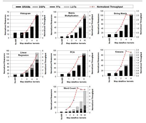
Fig. 7 Self performance-scalability tradeoff of HLSMapReduceFlow framework.
