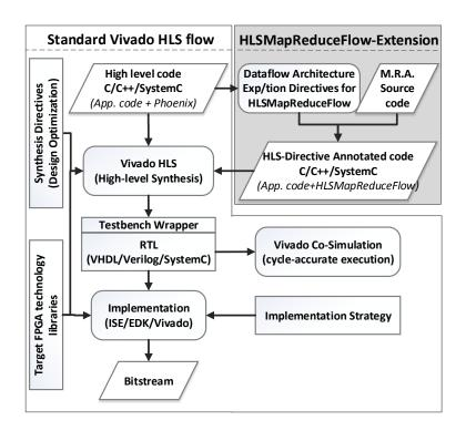
Fig. 4 Proposed extension on Vivado HLS flow to support MapReduce framework for FPGA-based systems.
