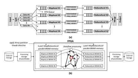
Fig. 2 HLSMapReduceFlow dataflow architecture: Every dataflow computation node is working in its unique memory. The system memory is partitioned to k-port and j-port banks for the k-map and j-reduce tasks respectively.
