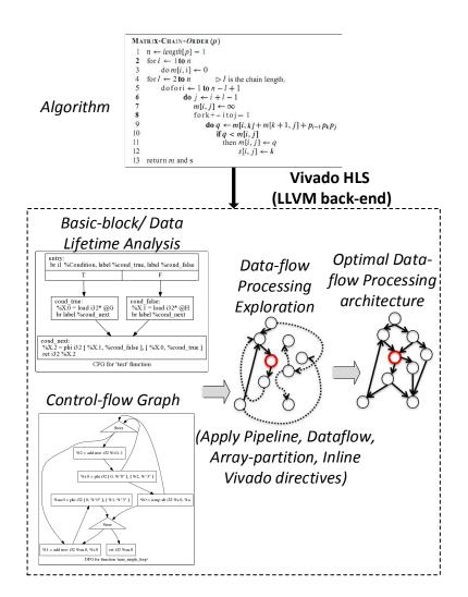
Fig. 3 Forcing data flow exploration from control-flow algorithm description with Vivado  $\rm HLS$
