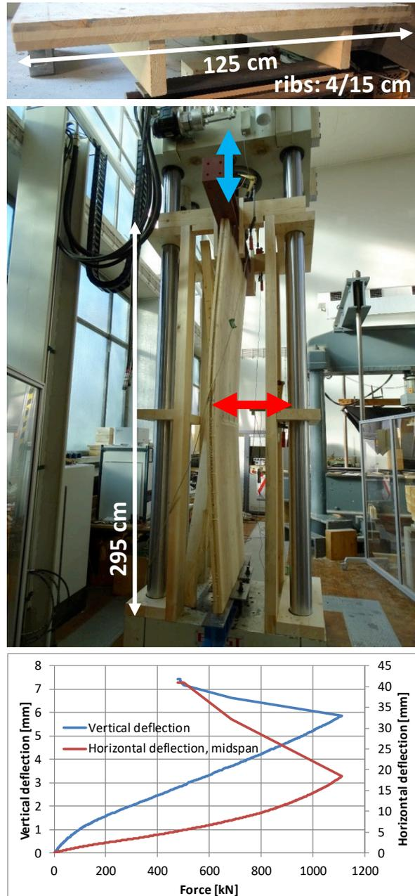
Figure 10: Load displacement curves for walls under in-plane compression loading
