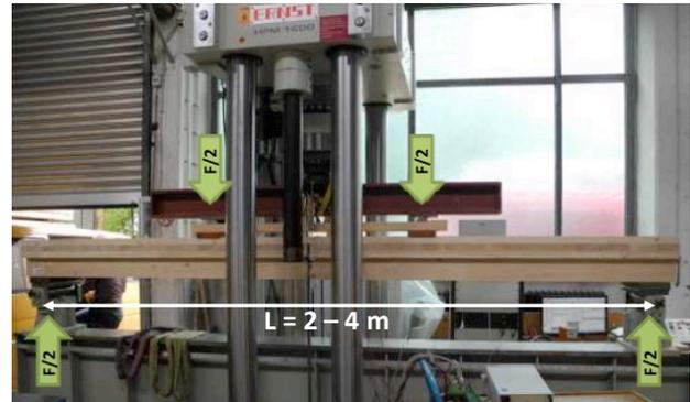
**Figure 7:** The 4-point bending setup
