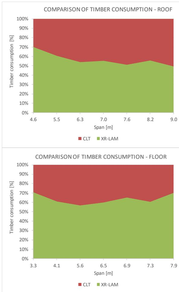
**Figure 12:** Comparison of timber use for floor and roof elements for conventional and ribbed CLT plates if calculated according to material characteristic values
