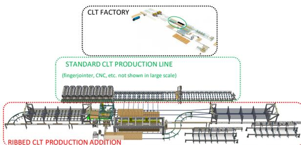
**Figure 13:** The XR-lam plate full industrial production line
